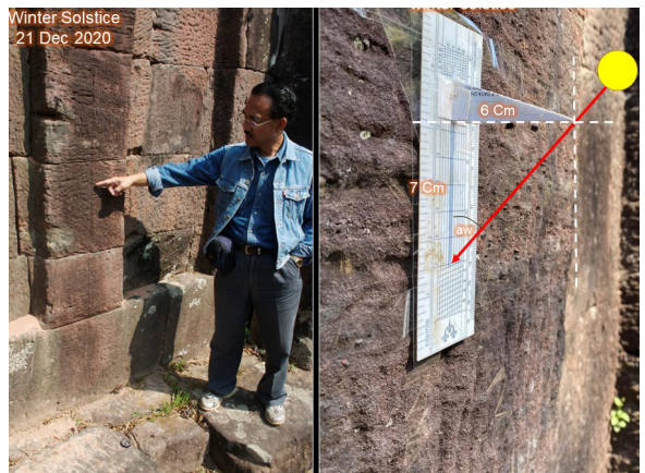
Figure 9. Placed the Sundial on the Wall of the South Door. In the Morning, the Sun's Shadow Points to the West. The Sun's Shadow at Solar Noon Pointed Directly to the Mark on the Sandstone Wall.
